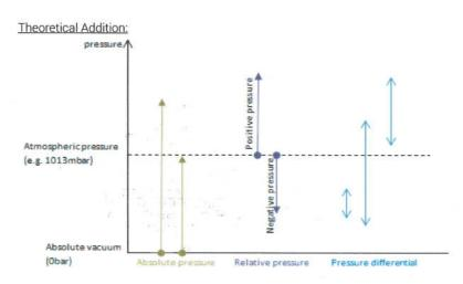
The absolute pressure is defined as the pressure which occurs with the absolute vacuum (0bar) as basis. At sea-level the absolute pressure is the same like the atmospheric pressure (1013mbar).
